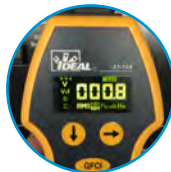
Displays neutral to ground voltage
