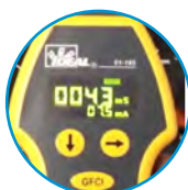
Trips GFCI at 6mA or 30mA
