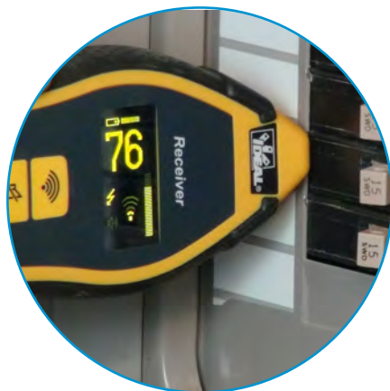
Finding Breakers or Fuses
