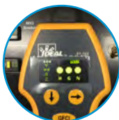
Displays H N G polarity
